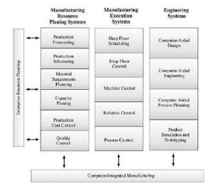
Manufacturing information systems help companies simplify, automate, and integrate many of the activities needed to produce products of all kinds. For example, computers are used to help engineers design better products using both computer-aided engineering (CAE) and computer-aided design (CAD) systems and achieve better production processes with computer-aided process planning. They are also used to help plan the types of material in the production
